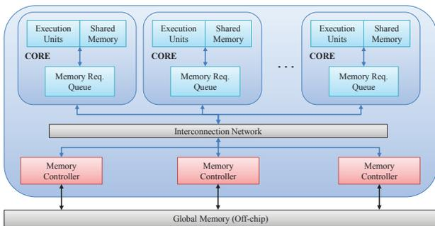
Figure 1. An overview of the baseline GPGPU architecture.
