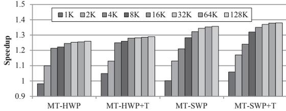
Figure 16. Sensitivity to prefetch cache size (+T: Throttling).
