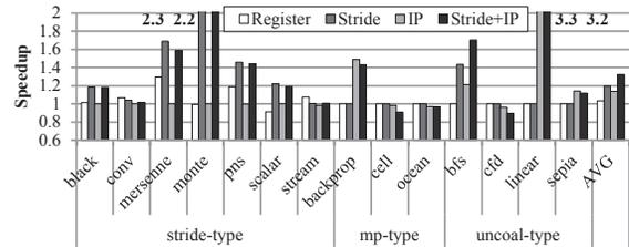
Figure 10. Performance of software GPGPU prefetching.
